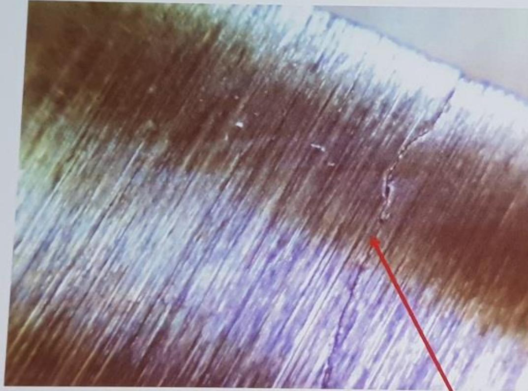
To the naked eye, this crack appeared to be only a small scratch in the finish of the instrument. However, upon closer examination this critical failure in the instrument integrity was found.
