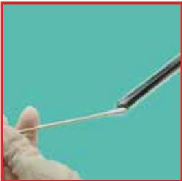
Cleaning the lens of an endoscope
