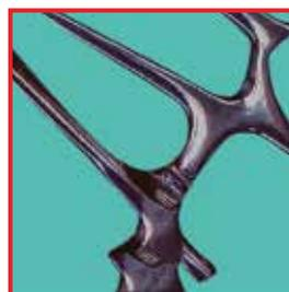
Retractors with discolored black shaft in hardened Cr-steel with the handle and blade remaining bright, made from non-hardenable CrNi steel.
