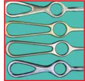
Titanium oxide discoloration occurs mostly on reflective surfaces over large surfaces, yellow-brown to blue-violet, sometimes with a shimmering appearance, in the wash chamber or over the entire surface of the instrument during machine-cleaning.
