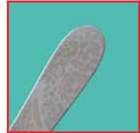
Typical silicate discoloration occurs, regardless of the nature of the surface, over large surfaces, yellow-brown to blue-violet in the cleaning & disinfection process, or in spots, droplet-shaped with pronounced condensation stain-like appearance during the steam sterilization process.
