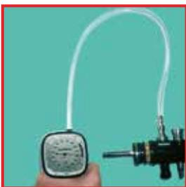
Manual leak test on flexible endoscope
