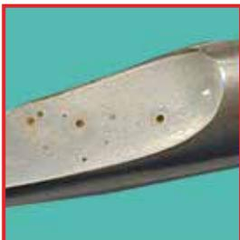
Chloride-induced pitting on instrument.
