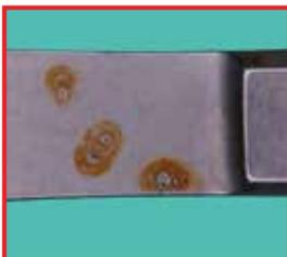
Tweeters in detail: Transition between spring and grip surface. Reactivation salt containing chloride caused massive pitting on the surface of the instrument. Leaking ion-exchanger connection in the W/D.
