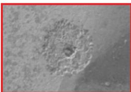
Scanning electron microscope image, chloride-induced pitting
