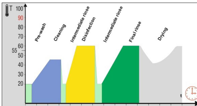
Cleaning program with chemo-thermal disinfection for heat-sensitive endoscopes
