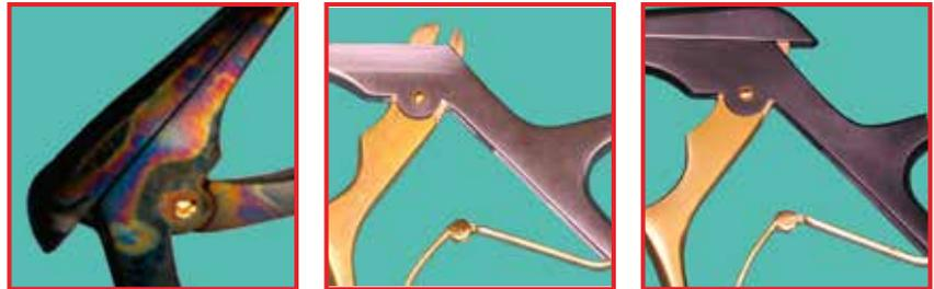
Example: black, TiAlN coated punch. The partial erosion of the layer has caused bright, colorful discoloration or complete removal of the layer with undamaged gold-plated components.
