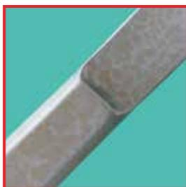
Stain pattern caused by silicic acid in steam condensation.
