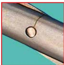
Stress cracks next to scissor hinge
