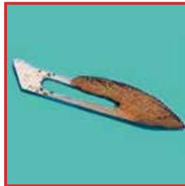
Surface of blade affected due to humidity. Cause: Composition of materials, normal steel, so disposable product.
