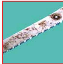
Material affected at partially defective chrome coating. Cause: Humidity causes corrosion to form on unprotected carrier material (normal steel)
