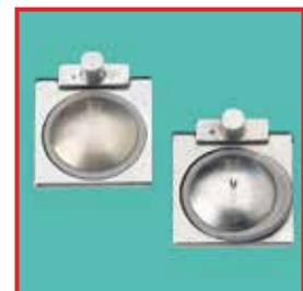
Right: Leaking flap valve on a trocar caused by the seal swelling as a consequence of contact with oil.
