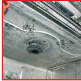
Rinsing chamber with heavy limescale deposits
