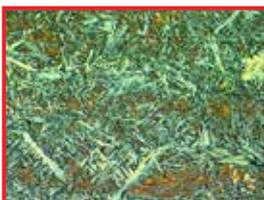
Color etching – martensitic structure (500x magnification)
