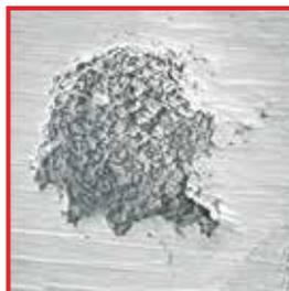
Pitting - seen under a scanning electron microscope
