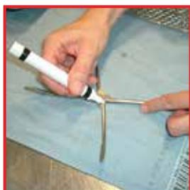
Maintenance or care means targeted application of instrument milk to the joints, hinges, locks, threads or friction surfaces of instruments such as clamps, scissors or punches, after they have been carefully cleaned and disinfected.
