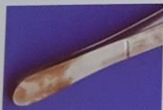
Crevice corrosion - Chemical residues - Insufficient drying
