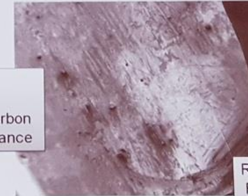
REM-Picture: deep Pitting Corrosion
